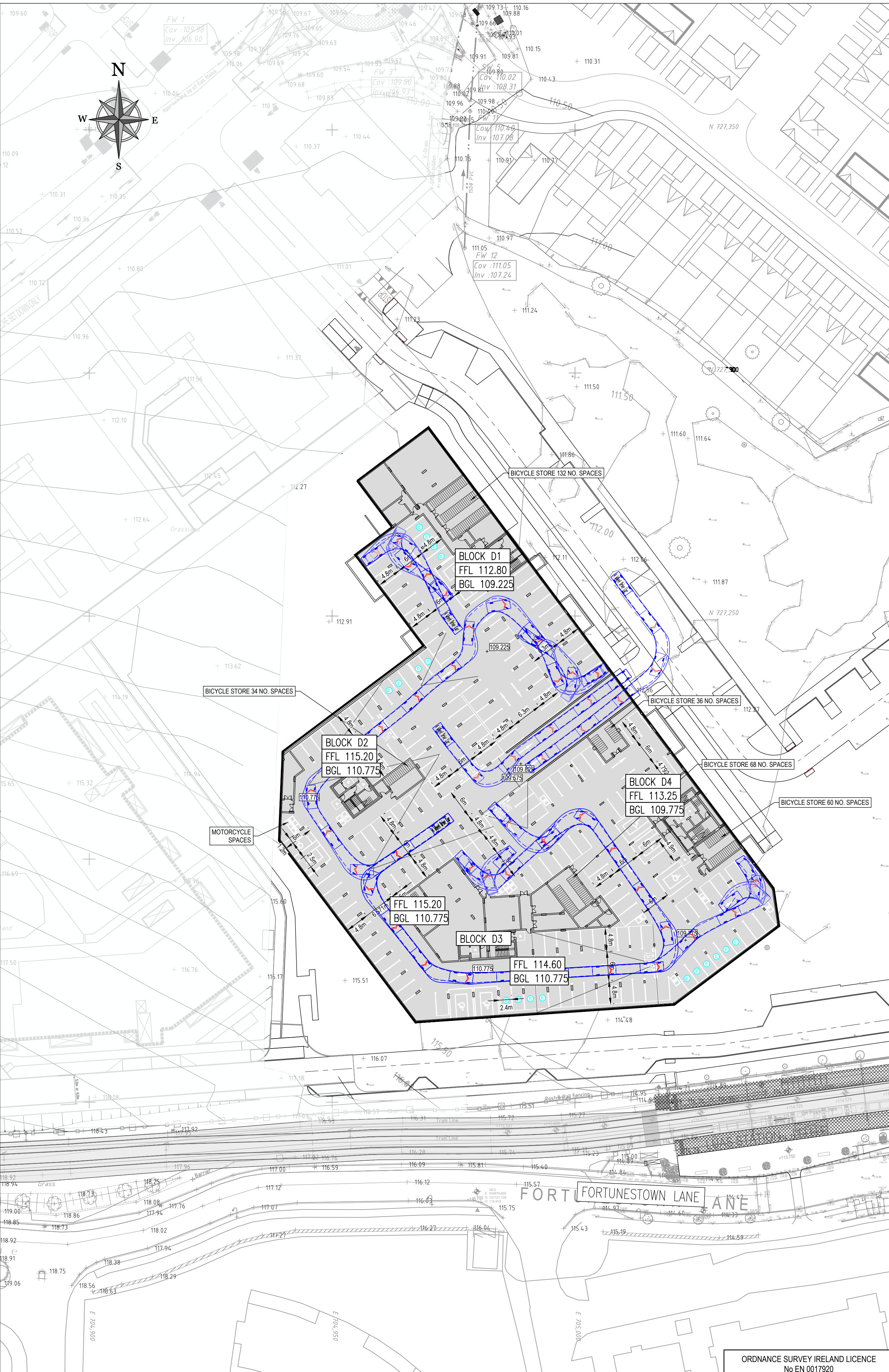
BASEMENT SWEEP PATH ANALYSIS
